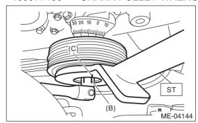
(4) Use the ST to lock the crank pulley, and tighten the crank pulley bolt to the angle where reference line (A) and end line (C) are aligned.
