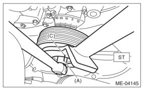
5) Install the V-belts. <Ref. to ME(H4DOTC)-37, INSTALLATION, V-belt.>
