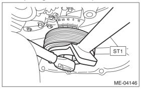
(3) Set the ST2, use the ST1 to lock the crank pulley, and tighten the crank pulley bolt to the specified angle.
