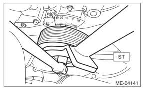
3) Remove the crank pulley.
