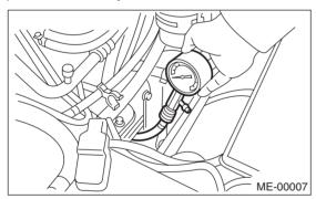
10) Perform at least two measurements per cylinder, and make sure that the values are correct.
