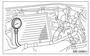
Vacuum pressure (at idling, A/C "OFF" ): Less than –60.0 kPa (–450 mmHg, –17.72 in-Hg)
