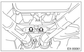
5) Install the nuts to cylinder head which hold front exhaust pipe.
