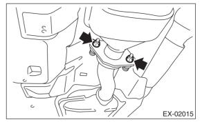
8) Tighten the bolts which hold front exhaust pipe assembly to hanger bracket.
