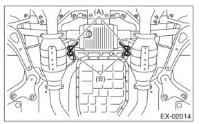
5) Separate the front exhaust pipe from the rear exhaust pipe.
