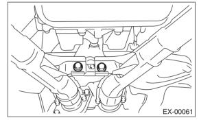
8) Remove the front exhaust pipe assembly from vehicle.
