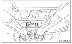
9) Connect the front oxygen (A/F) sensor connector (A) and rear oxygen sensor connector (B).
