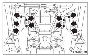
7) Remove the bolts which hold front exhaust pipe assembly to hanger bracket.
