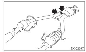
10) Remove the front oxygen (A/F) sensor and rear oxygen sensor. <Ref. to FU(H6DO)-29, REMOV-AL, Front Oxygen (A/F) Sensor.> <Ref. to FU(H6DO)-31, REMOVAL, Rear Oxygen Sensor.>
