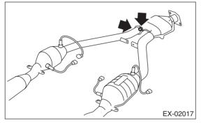
3) Install the front exhaust pipe assembly to vehicle.
