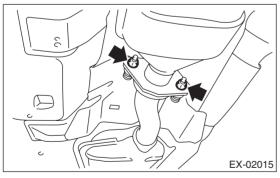
6) Remove the nuts which hold front exhaust pipe onto cylinder heads.
