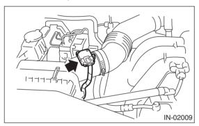
3) Remove the mass air flow and intake air temperature sensor.
