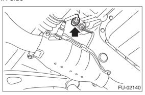
5) Remove the front oxygen (A/F) sensor.
