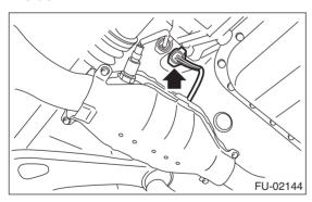
5) Remove the clip holding the harness.
