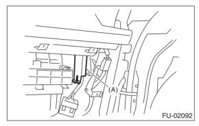
4) Disconnect the connector from electric throttle control relay.
