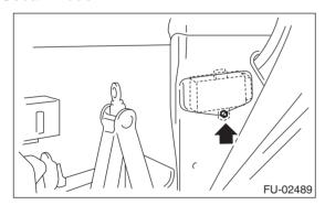
4) Disconnect the connector from fuel pump control unit.
