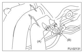
4) Remove the manifold absolute pressure sensor from intake manifold.
