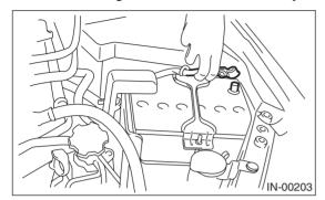
3) Disconnect the connector from manifold absolute pressure sensor (A), and remove the filter assembly (B) from intake manifold.
