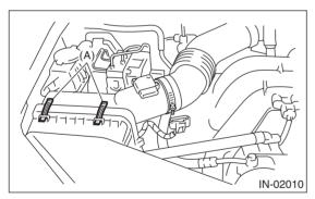
4) Pull the air cleaner case (rear) backward of the vehicle, and remove the air cleaner element.
