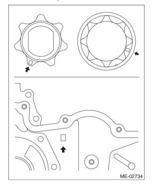
• When replacing any one of inner rotor, outer rotor and rear chain cover with new part Select suitable size from following table so that side clearance is standard.
