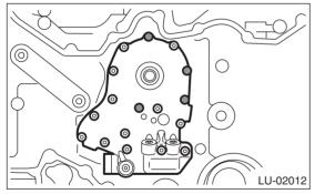
13) Remove the inner rotor and outer rotor.
