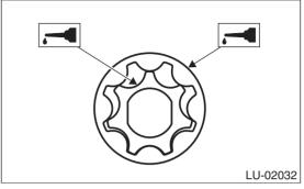
2) Set the inner rotor onto opening edge of crank shaft, and install the inner rotor, and then assemble the outer rotor.
