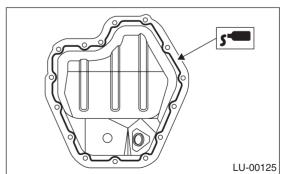
3) Tighten the oil pan lower installing bolts in the numerical order as shown in the figure.
