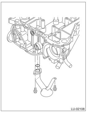
2) Apply liquid gasket to the mating surfaces, and install the oil pan.
