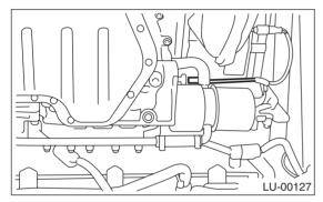
6) Remove the oil pressure switch.
