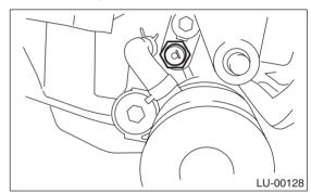
3) Connect the terminal of the oil pressure switch.
