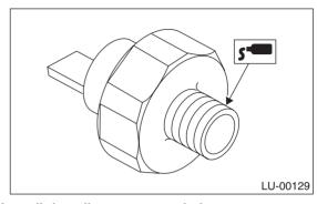
2) Install the oil pressure switch.
