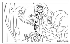
9) Perform at least two measurements per cylinder, and make sure that the values are correct.
