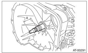
4) While holding the torque converter assembly by hand, carefully install it to the converter case. Take care not to damage the bushing. Do not allow the oil pump shaft bushing to touch the starter shaft part of the oil pump cover inappropriately.
