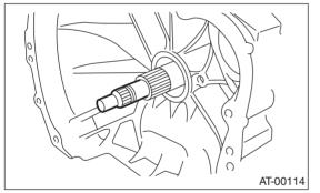
4) Remove the oil pump shaft from torque converter assembly as necessary.
