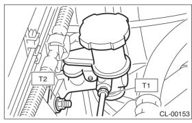
2) Connect the push rod of the master cylinder to the clutch pedal, and install the clevis pin and snap pin.
