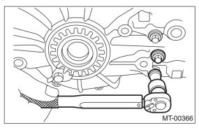
10) Install the differential assembly. <Ref. to 5MT-66, INSTALLATION, Front Differential Assembly.> 11) Install the main shaft assembly.
