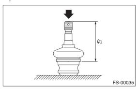
(2) With 686 N (70 kgf, 154 lb) loaded in direction shown in the figure, measure the length  $\varrho_2$ .
