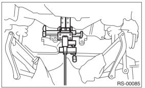
7) Remove the front link from sub frame.
