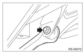
4) Remove the bolt which secures the front link to rear arm, then remove the front link.
