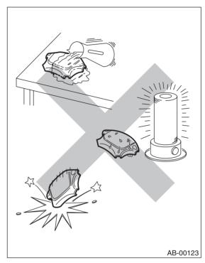
• After removal of each parts for airbag system, keep them with the pad facing upward on a dry, clean and flat surface without heat, light sources, moisture and dust.
