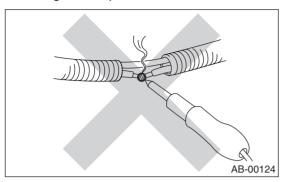
• Install the wiring harness securely with specified clips to avoid interference or becoming tangled with other parts.
