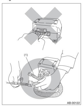
• Do not allow water or oil to come in contact with the connector terminals. Also, do not touch the connector terminals.
