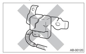
• When checking the airbag system, be sure to use a digital circuit tester. Use of an analog circuit tester may cause the airbag to activate erroneously due to a minimal current inside tester.
