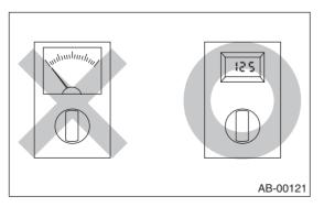
• When checking, use a test harness (1). Damage to connector terminal cause malfunction. Do not directly apply the tester probe to connector terminal of airbag.
