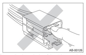
Do not check continuity of the airbag modules for driver's side, passenger's side and curtain, or the pretensioner.
