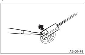
(2) Pull the connector to disconnect from the driver's airbag module assembly or the retractor assembly.
