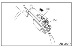
(3) With the slide lock held in the moved position, release the lock arm (return to original position) and disconnect the connector.
