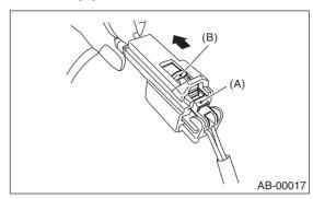
(3) With the slide lock moved, release the lock arm (return to original position) and disconnect the connector.
