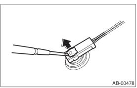
(2) Pull the connector to disconnect from driver's airbag module assembly or retractor assembly.
