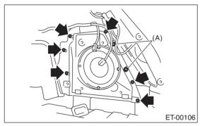
5) Disconnect the harness connector and detach the woofers.
