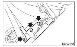
3) Remove clamp (A) of the window washer hose, and remove the bolt of the hinge.
