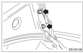
Remove the clip, and remove the cowl side panel front.
