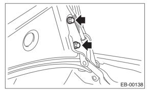
3) Adjust the height at the front end of hood. <Ref. to SL-46, ADJUSTMENT, Front Hood Lock Assembly.>
