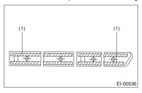
Double-sided tape: thickness 1.2 mm (0.047 in), width 5mm (0.197 in)
