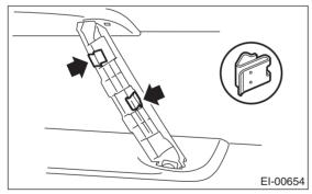
• Lower side of the hand grip cover for the front door has a claw.
