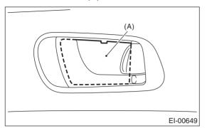
3) Push the root of hand grip upward, and remove the hand grip cover by twisting it towards the front of the vehicle.
