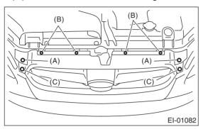
3) Pull the lower side of the front grille forward, remove hooks (A), and then remove the front grille from vehicle body.
