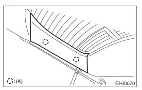
2) Remove the clips, and remove the rear gate upper trim.
