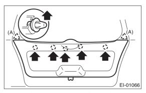
6) Remove the rear gate weather strip.
