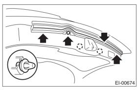
5) Remove the clips (A), and remove the rear gate lower trim.
