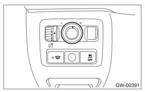
3) Remove the remote control mirror switch from instrument panel lower cover.
