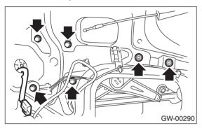
5) Remove the screws to remove motor assembly.
