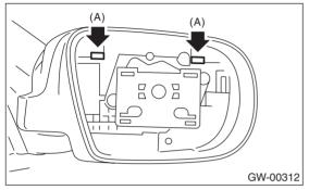
3) Pull the scalp cap frontward of outer mirror, remove the upper side clips (A) and lower side hooks (B), and then remove the scalp cap.
