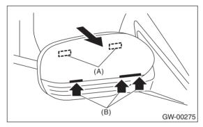
4) Insert the lower hooks (B) of scalp cap to the outer mirror and push the upper clips (A) in.
