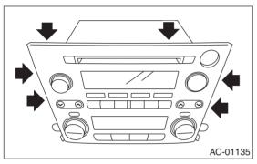
3) Use a fine flat tip screwdriver to lift the hooks in 10 locations gradually. Starting from the sides, proceed to loosen the lower hooks, then the upper hooks, then remove.
