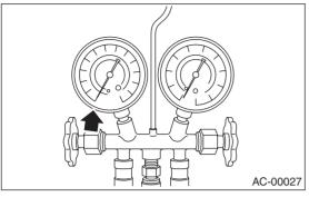
8) Leave it at least 5 minutes, and then check the low-pressure gauge reading for any changes. If the gauge indicator shows near zero point, it is a sign of leakage. Check pipe connector points, repair them, and make sure there is no leakage.9) Follow the can tap operation manual, install to the refrigerant can.
