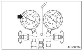
24) Adjust the refrigerant flow to maintain the pressure on the low-pressure side at 276 kPa (2.81 kg/  $cm^2$ , 40 psi) max.
