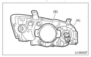
7) Remove the light bulb retaining spring (A) to remove bulb.
