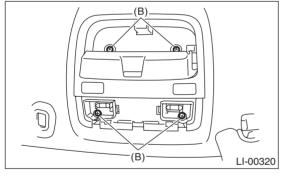
3) Disconnect the harness connectors and remove the spot map light.
