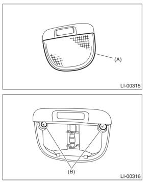
3) Disconnect the harness connector and remove the room light.
