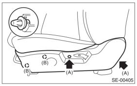
5) Loosen the screws to detach the seat side cover inside.
