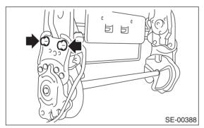
17) Remove the hog rings (A) on the surface side of backrest, and then remove the backrest cover from backrest.
