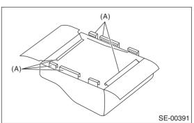
19) Remove the hog rings (A), and then remove the seat cushion cover from seat cushion pad.
