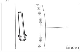
10) Remove the hooks and hog rings at the rear side of backrest.
