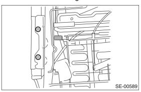
16) Remove the hog rings (A) on the surface side of backrest, and then remove the backrest cover from backrest.
