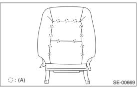
17) Remove the bolt (A) and hook (B) on left and right side, and then remove the seat cushion frame from seat rail assembly.
