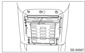
11) Remove the headrest lock bushing.
