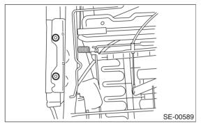
16) Remove the two bolts on each left and right side, and then remove the reclining motor assembly.
