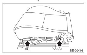
18) Remove the hooks (A), and then remove the seat cushion from seat cushion frame.
