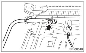
21) Remove the bolts, then remove the slide rail.
