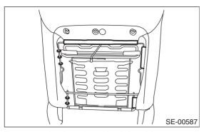
11) Remove the headrest lock bushing.
