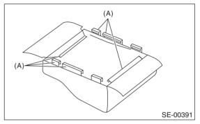
20) Remove the hog rings (A), and then remove the seat cushion cover from seat cushion pad.
