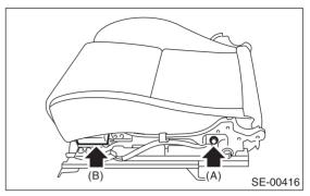
19) Remove the hooks (A), and then remove the seat cushion from seat cushion frame.
