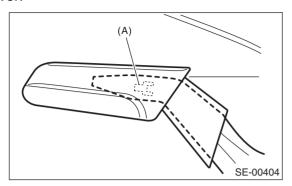
4) Remove screws (A) and clips (B), and then detach the seat side cover outside.
