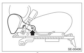
6) Remove the TORX<sup>®</sup> bolt, and then remove the inner seat belt assembly.
