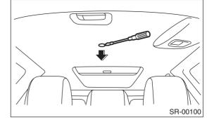
4) Insert the hexagon wrench securely until it touches the motor shaft edge.
