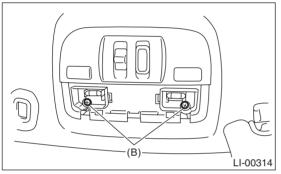
3) Disconnect the harness connector, and then remove the sunroof switch.
