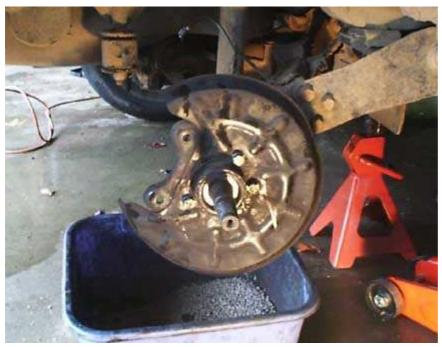
13. inspect the splines on the axle stub, and hub. They should be square on the tops, if they're
