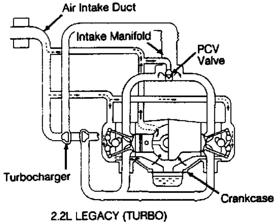
Fig. 21: Positive Crankcase Ventilation (PCV) Systems (Legacy Turbo)
