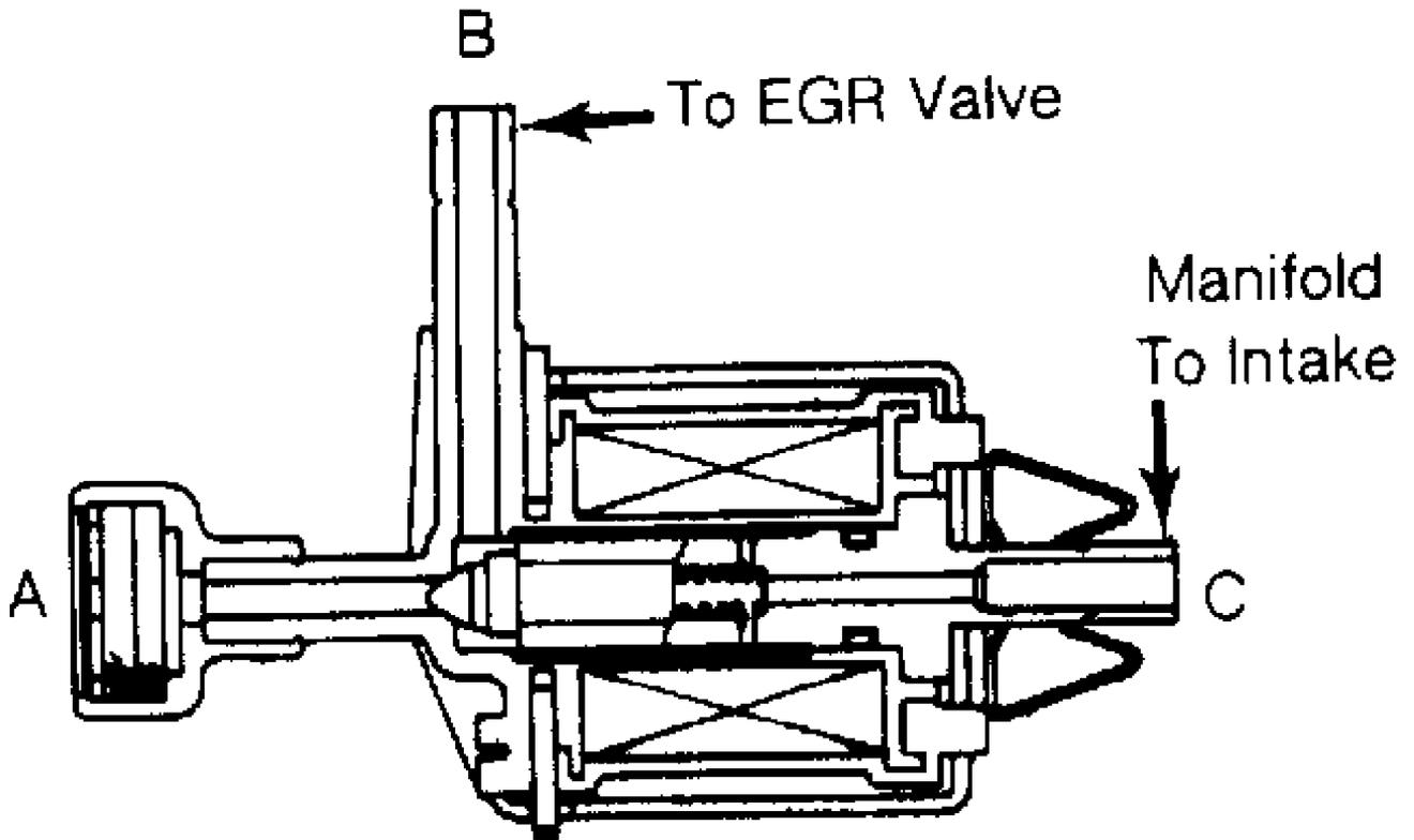
Fig. 9: Cross-Sectional View Of EGR Solenoid Valve
