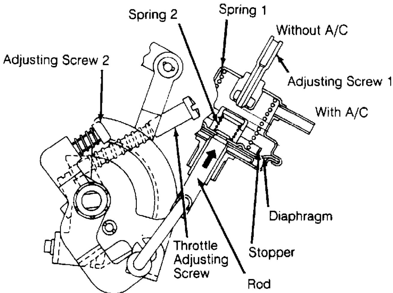
Fig. 1: Fast Idle Control Device (FICD) Control Actuator
