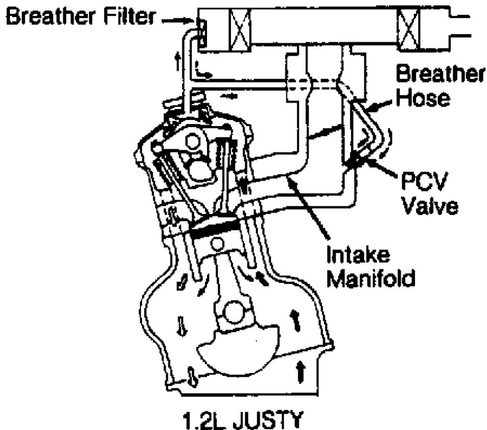
Fig. 18: Positive Crankcase Ventilation (PCV) Systems (Justy)
