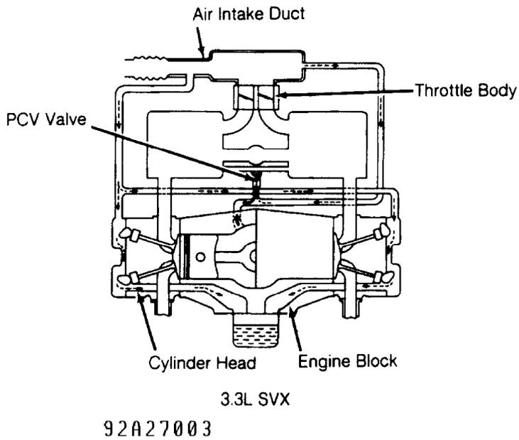
Fig. 22: Positive Crankcase Ventilation (PCV) Systems (SVX)
