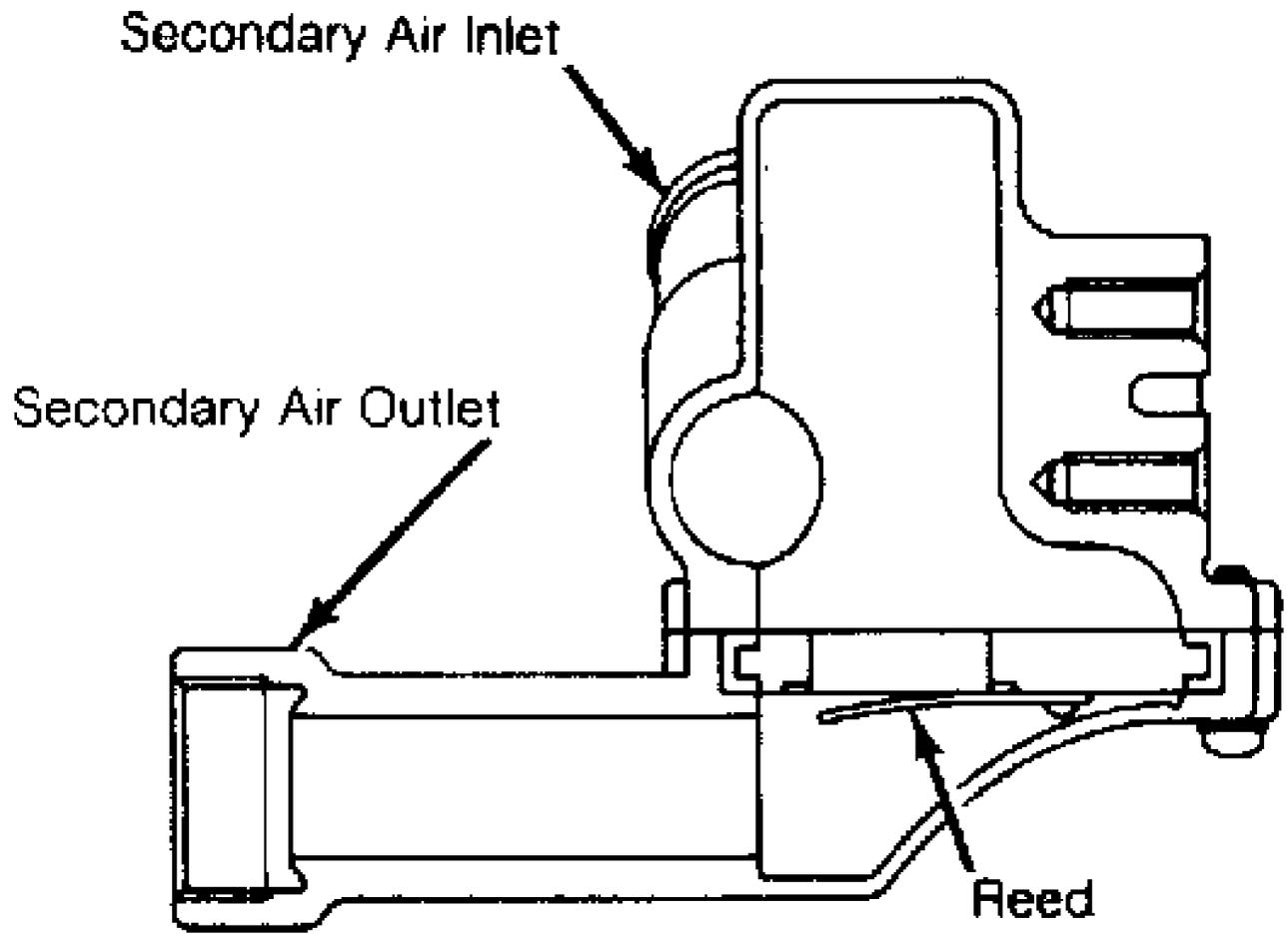
Fig. 4: Cross-Sectional View Of Suction Valve (Justy)
