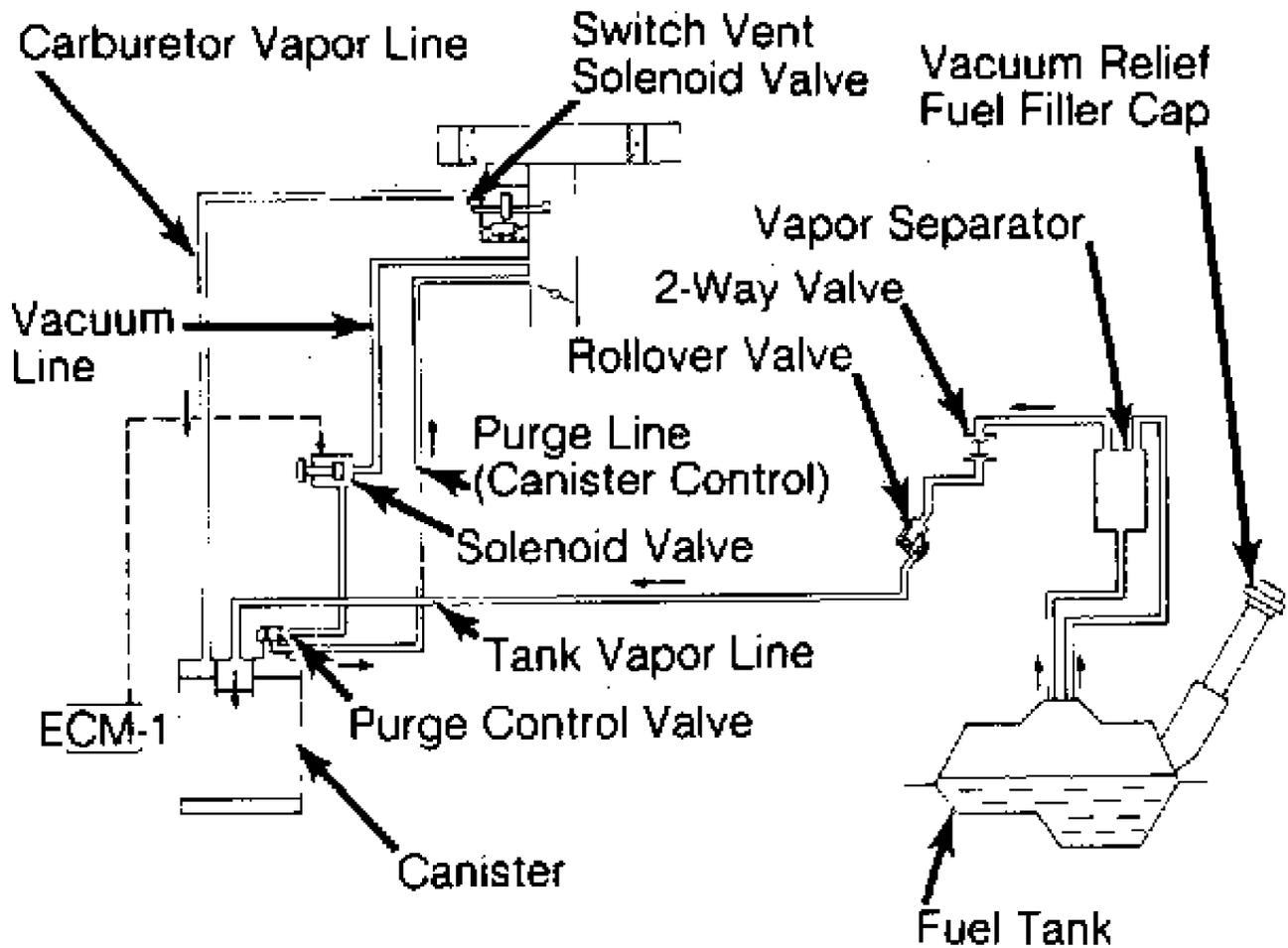
Fig. 10: Fuel Evaporation System (Justy)
