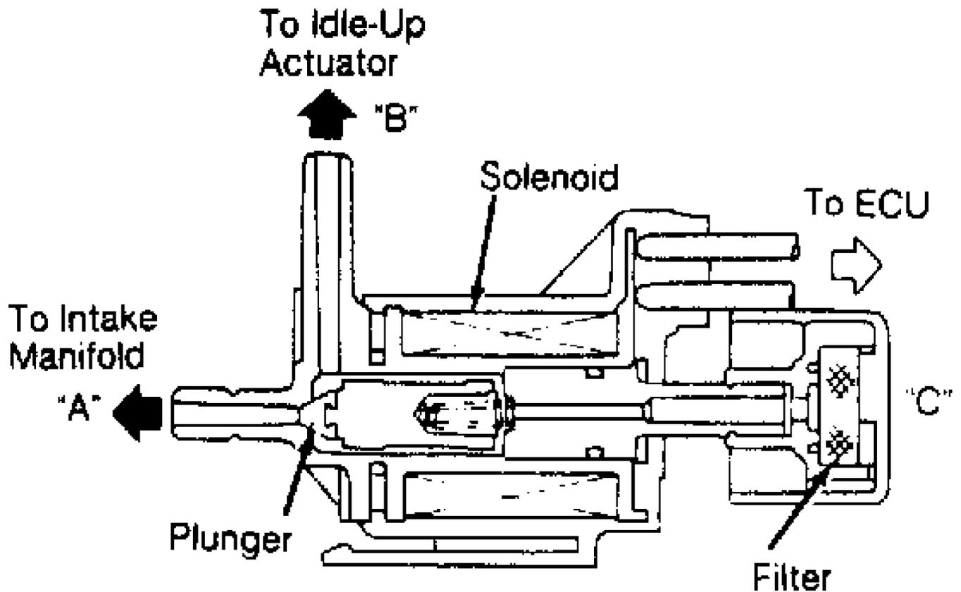
Fig. 2: Identifying Idle-Up Solenoid (Justy Carbureted)
