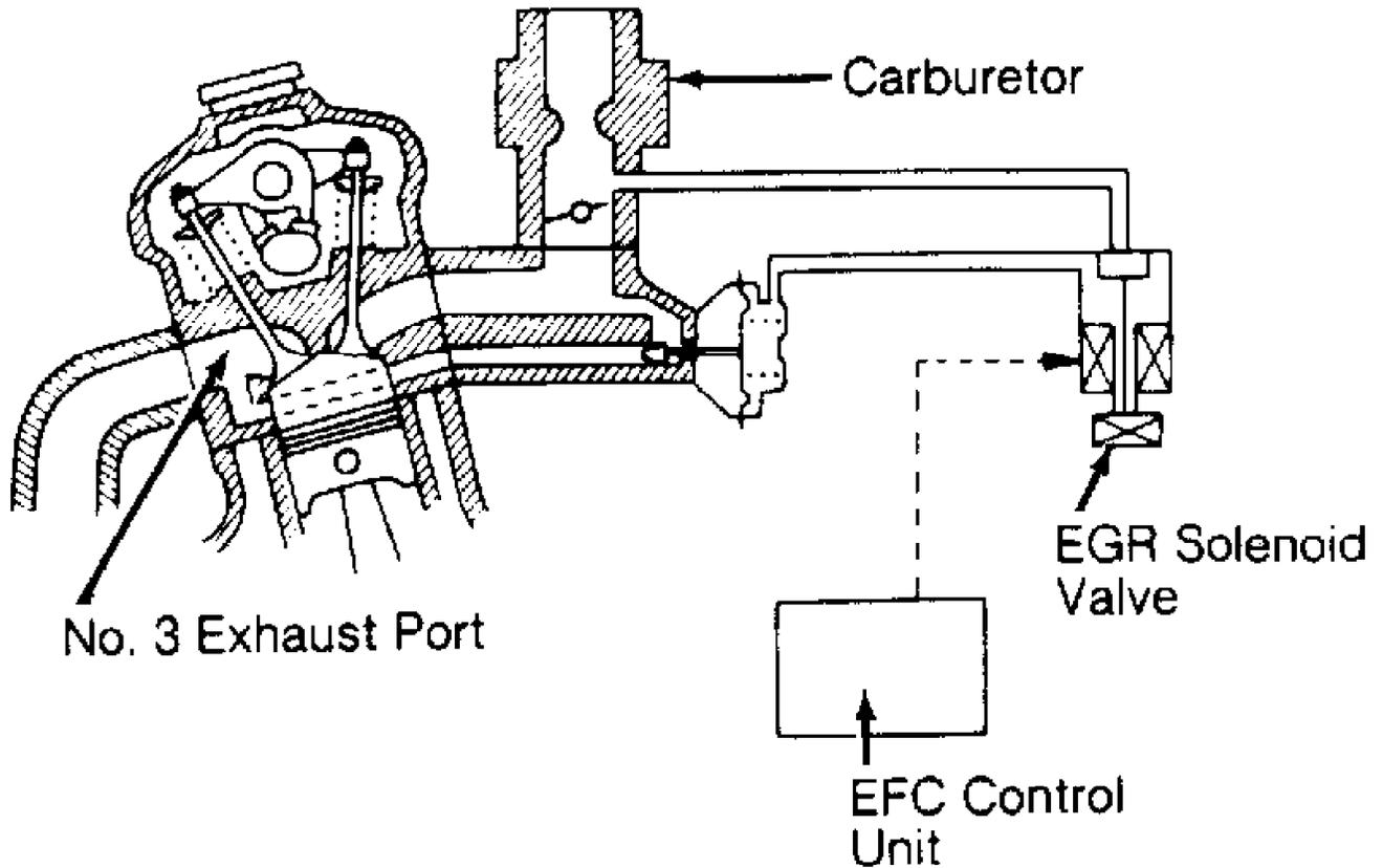
Fig. 6: EGR System (Justy Carbureted)
