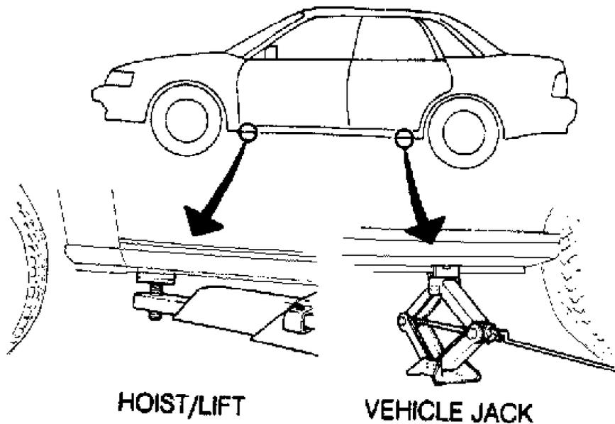
Fig. 1: Locating Hoisting/Lifting Points On Lower Body Seam
