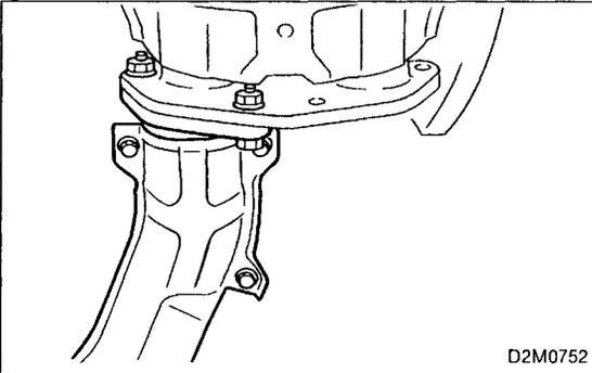
2) Install front exhaust pipe to rear catalytic converter.
