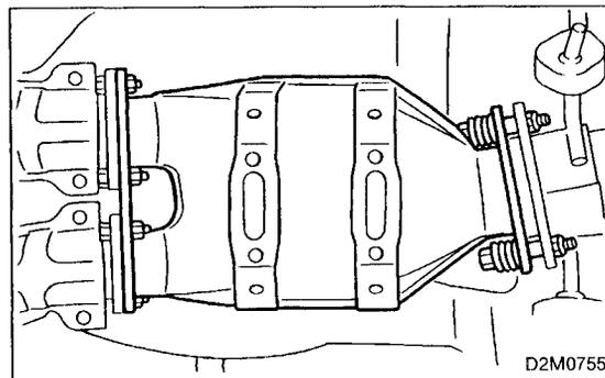
2) Install rear catalytic converter to front exhaust pipes.
