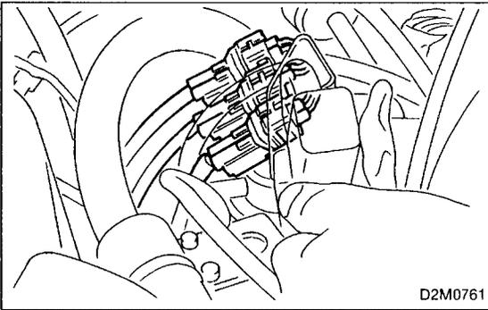
5) Disconnect ignition coil connectors (engine RH).
