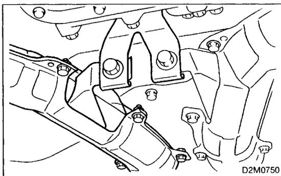
6) Remove front exhaust pipe from hanger bracket.
