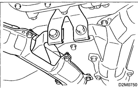
5) Tighten nuts which hold front exhaust pipes to hanger bracket.
