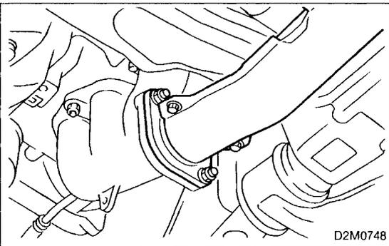
3) Install front exhaust pipe to exhaust manifold.
