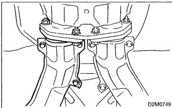
5) Separate front exhaust pipe from rear catalytic converter.
