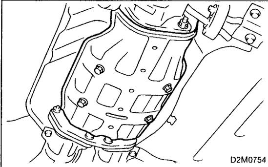
3) Install rear catalytic converter protector.
