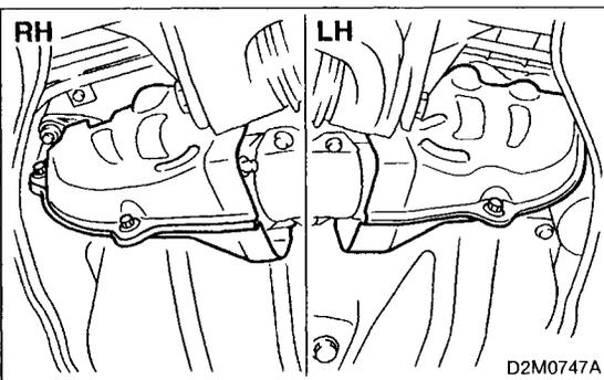
6) Install exhaust manifold covers (RH and LH).
