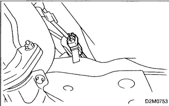
4) Connect rear oxygen sensor connector.
