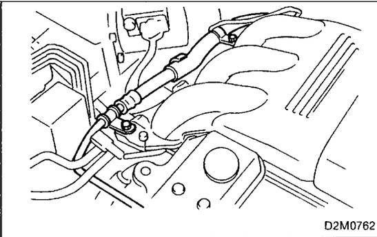
6) Remove bolts which install power steering hose bracket to engine, and position the hose away from engine.
