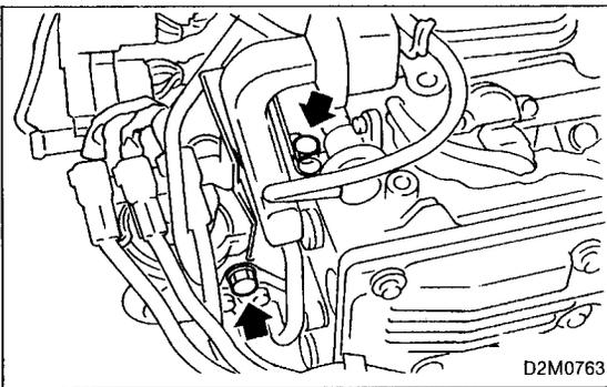
7) Remove bolts which install BPT bracket to cylinder block.
