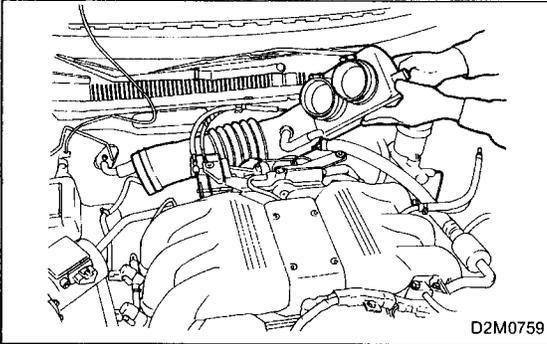
2) Remove air intake duct.
