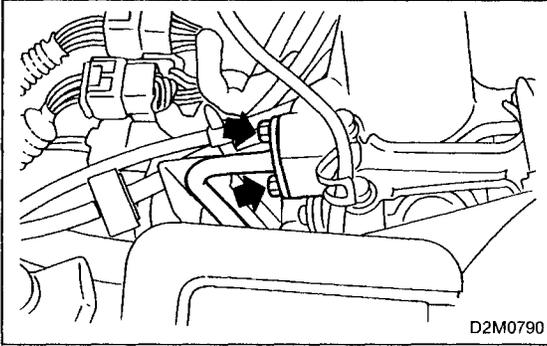
16) Remove EGR pipe cover, then remove bolts which install EGR pipe to collector chamber.
