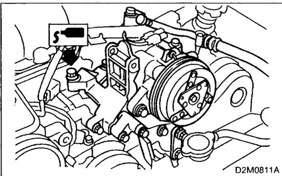
2) Install A/C compressor and bracket onto cylinder block.
