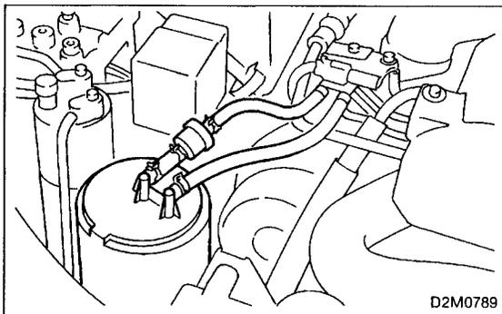
16) Connect canister hoses to evaporation pipes.
