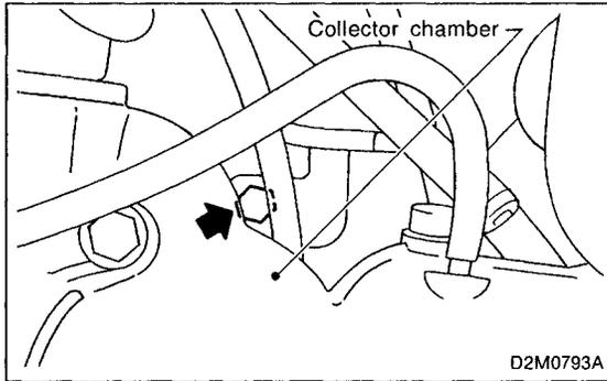
22) Remove bolt which installs fuel pipe to cylinder block.
