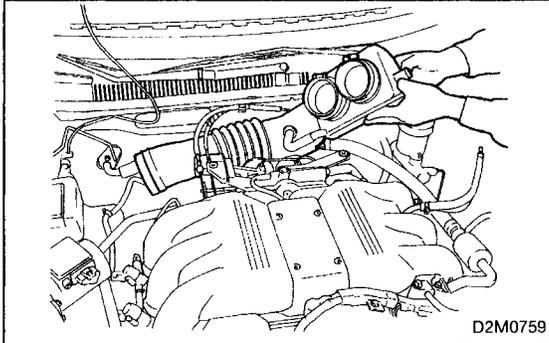
2) Loosen clamps which connect air intake duct to throttle body and mass air flow sensor.
