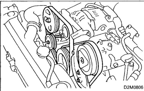
24) Remove V-belts from generator and A/C compressor.
