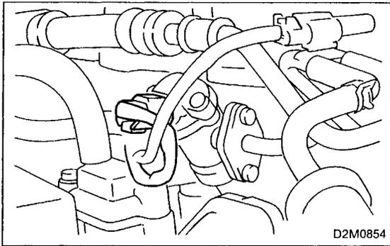
6) Disconnect connectors from each fuel injector.
