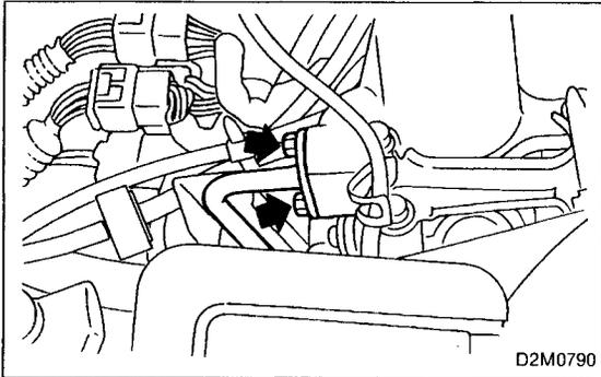
11) Install bolts which connect EGR pipe to collector chamber.
