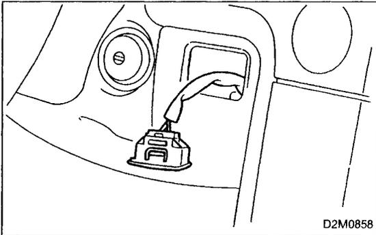
2) Pull out the data link connector from lower cover panel.
