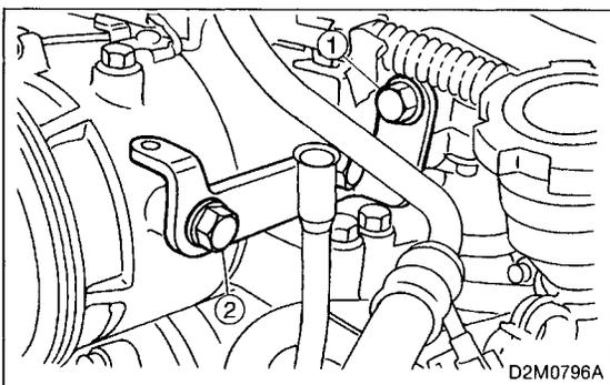
2) Install A/C bracket to collector chamber and tighten bolts ① and ②.
