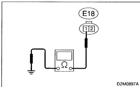
5) Measure resistance of harness between auxiliary air control valve connector and engine ground.
