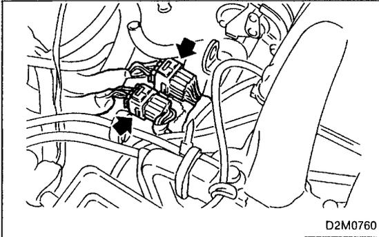
17) Disconnect engine harness connectors from bulkhead harness connectors.
