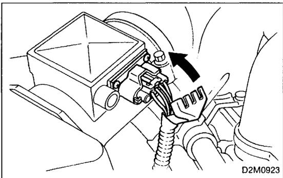
21) Connect connector to mass air flow sensor.
