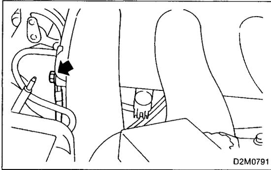
10) Install engine ground wire to collector chamber.
