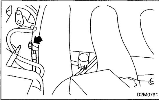
16) Remove engine ground wire from collector chamber.
