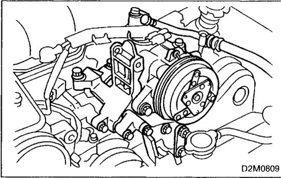
27) Remove A/C compressor with bracket, and move A/C compressor forward to facilitate removal of intake manifold mounting bolts.
