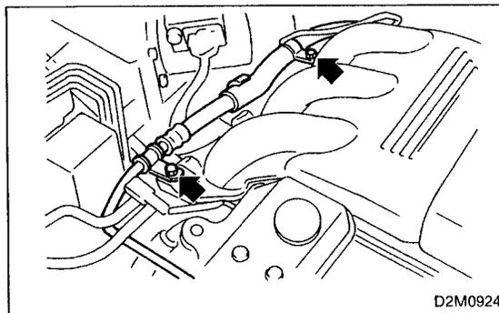
15) Install power steering hose bracket to collector chamber.
