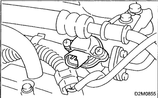
7) Remove screws which hold fuel injector to fuel injector pipe.
