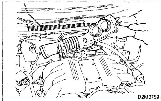
4) Loosen clamps which connect air intake duct to throttle body and mass air flow sensor.
