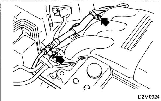
13) Install power steering hose bracket to collector chamber.
