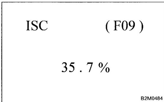
17) After the engine has warmed up, read the idle air control solenoid valve duty ratio using Subaru select monitor. At this point, the engine must be under no load (radiator fan, A/C, headlights and accessories switches are all OFF).
