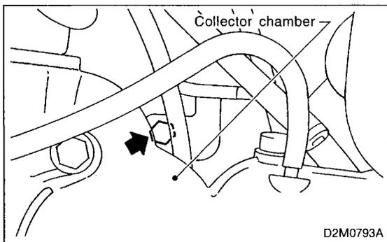
6) Install bolt which holds fuel pipe on cylinder block.
