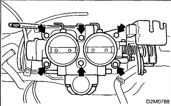
9) Remove bolts which install throttle body to collector chamber.
