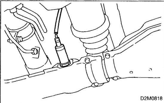
2) Install front oxygen sensor 1.
