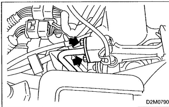
13) Install bolts which connect EGR pipe to collector chamber.
