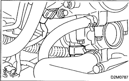
8) Disconnect connectors from throttle position sensor and idle air control solenoid valve.
