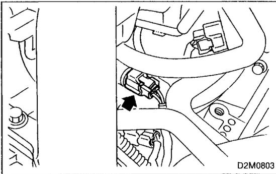
19) Disconnect connector from auxiliary air control valve.
