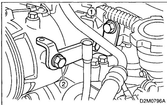
25) Remove bolt ① which installs A/C bracket to collector chamber, then loosen bolt ②.
