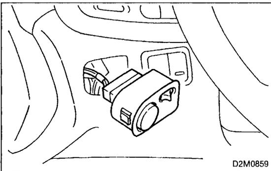
3) Pull out the remote control rearview mirror switch, and disconnect connector from it.
