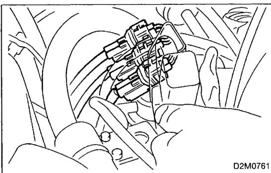
19) Disconnect ignition coil connectors (engine RH).
