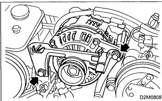
26) Remove bolts which install generator to bracket, then remove generator.
