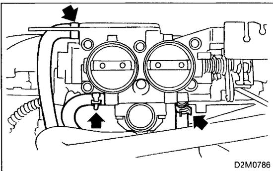
15) Connect engine coolant hoses and air hose to throttle body.
