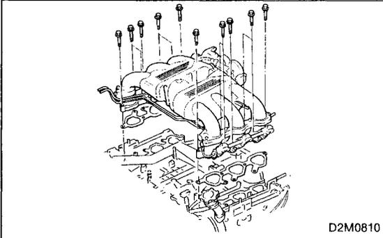
28) Remove bolts which hold intake manifolds onto cylinder heads.
