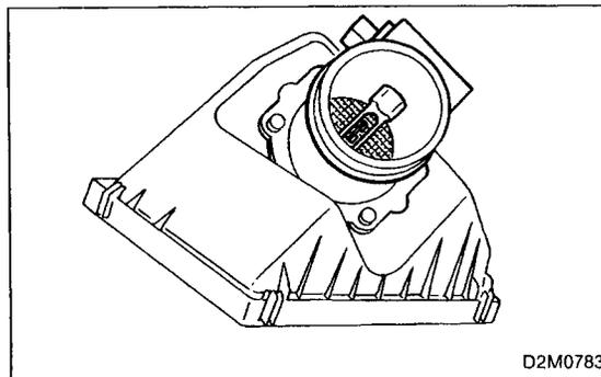
7) Remove mass air flow sensor from air cleaner upper cover.
