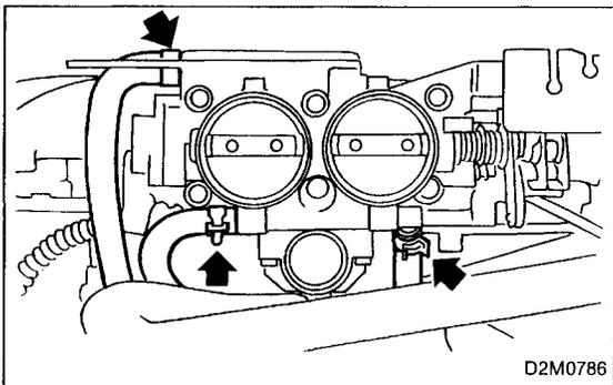
17) Connect engine coolant hoses and air hose to throttle body.
