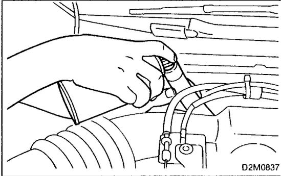
12) While operating the engine in the 1,500 — 2,000 rpm range, spray the cleaner from the air by-pass hose on the idle air control valve for 10 seconds.
