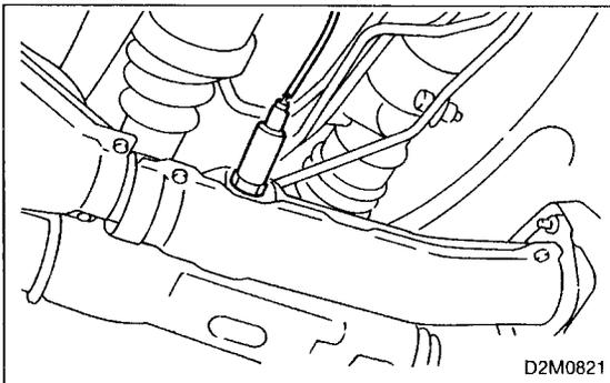
2) Install front oxygen sensor 2.
