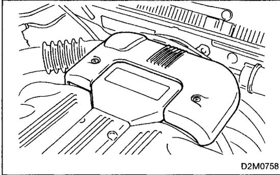
**1. Air Cleaner and Air Intake Duct****A: REMOVAL AND INSTALLATION**
