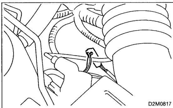
**9. Front Oxygen Sensor 1 (RH)****A: REMOVAL**
