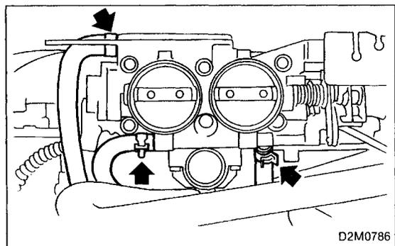
7) Disconnect engine coolant hoses and air hose from throttle body.
