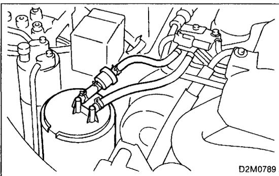
14) Connect canister hoses to evaporation pipes.
