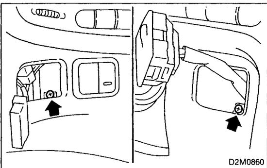
4) Remove bolts which install lower cover panel.
