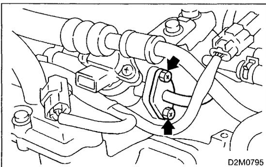
3) Install and tighten bolts which connect fuel pipes to fuel injector pipes.
