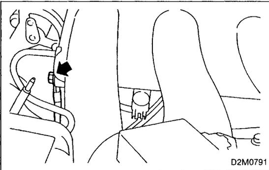
17) Remove engine ground wire from collector chamber.
