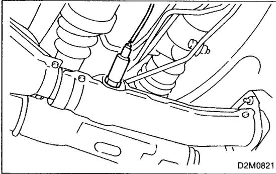
4) Remove front oxygen sensor 2.
