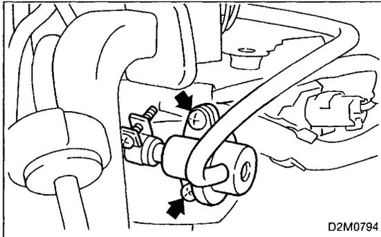
23) Remove pressure regulator from fuel injector pipe.
