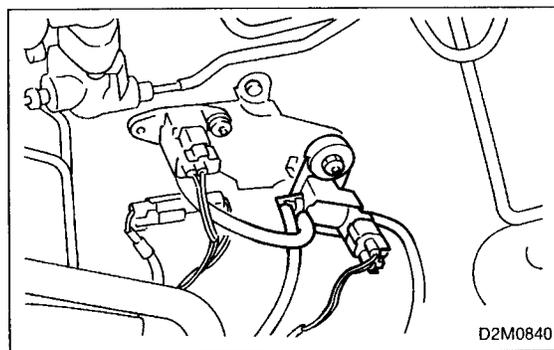
**16. Pressure Sources Switching Solenoid Valve**
