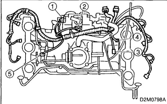
4) Attach engine harness to collector chamber.
