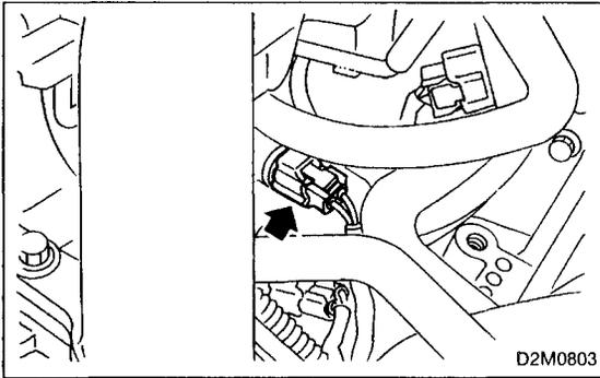
9) Connect connector to auxiliary air control valve.
