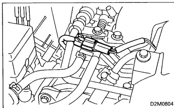
8) Connect power steering switch connector.
