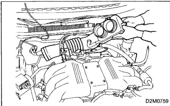
23) Install air intake duct, and tighten it with clamps.
