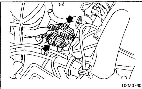
18) Disconnect engine harness connectors from bulk-head harness connectors.
