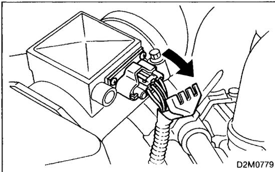
4) Slide connector cover out from mass air flow sensor connector.
