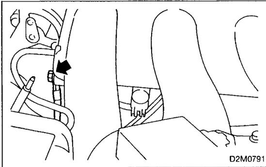
12) Install engine ground wire to collector chamber.
