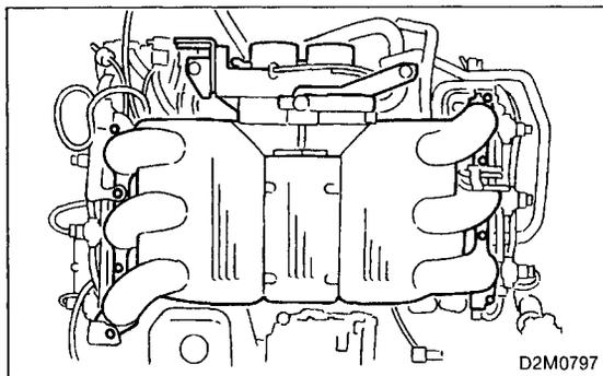
26) Remove bolts which hold collector chamber onto intake manifolds.
