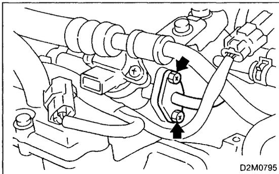
24) Remove bolts which install fuel pipes to fuel injector pipes.
