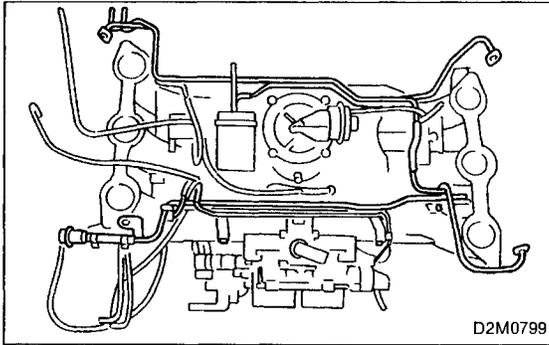
3) Install fuel pipes to collector chamber.
