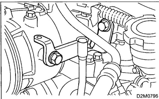
3) Install A/C bracket to collector chamber.
