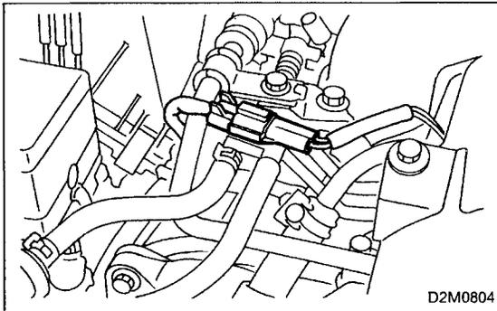
20) Disconnect power steering switch connector.
