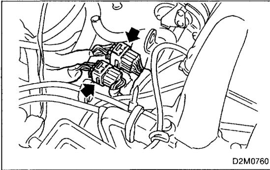
10) Install bulkhead harness connectors to bracket.
