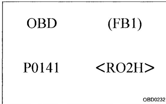
**O: DTC P0141****— REAR OXYGEN SENSOR HEATER CIRCUIT MALFUNCTION (RO2H) —****DTC DETECTING CONDITION:**
