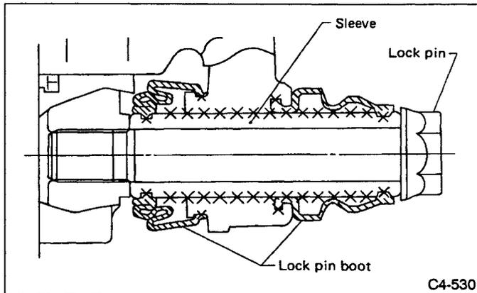
Fig. 58 Grease application to lock pin portion
