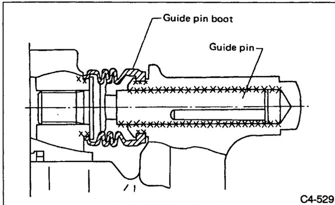
Fig. 57 Grease application to guide pin portion
