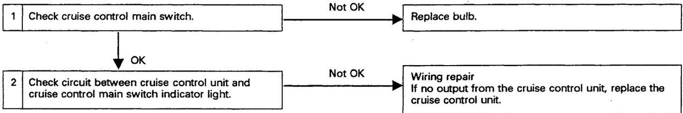
**1. CHECKING THE INDICATOR LIGHT IN THE CRUISE CONTROL MAIN SWITCH**
